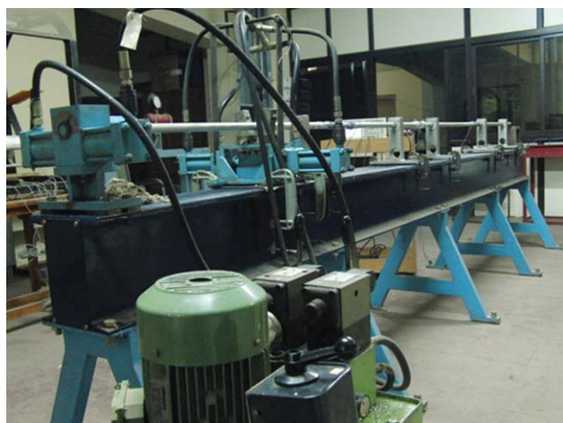
Figure 1 Photograph of TSHB apparatus. [Color figure can be viewed in the online issue, which is available at wileyonlinelibrary.com .]
